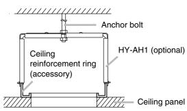
**Step 4.** Attach a safety wire to prevent the speaker from accidentally falling.
