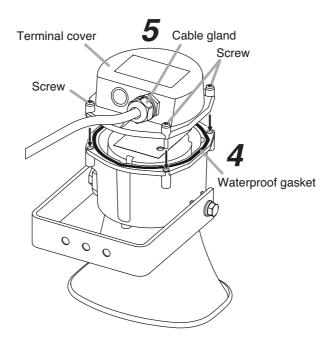
Step 5. Securely tighten the cable gland.
