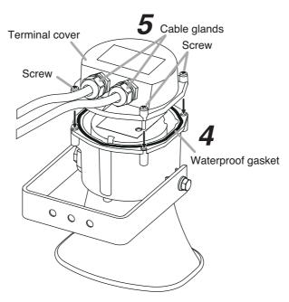
Step 7. Securely tighten the cable glands.
