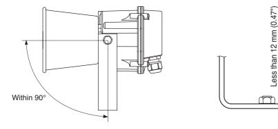
• Do not install the speaker face-up from a horizontal plane. If water accumulates in the horn, this may cause the speaker malfunction.
