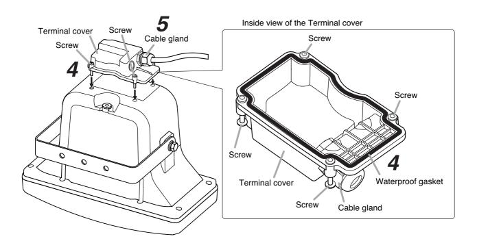
Step 5. Securely tighten the cable gland.
