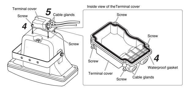
Step 7. Securely tighten the cable glands.
