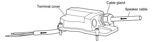
Step 3. Connect the speaker cable according to the polarity indication at the screw terminal.
