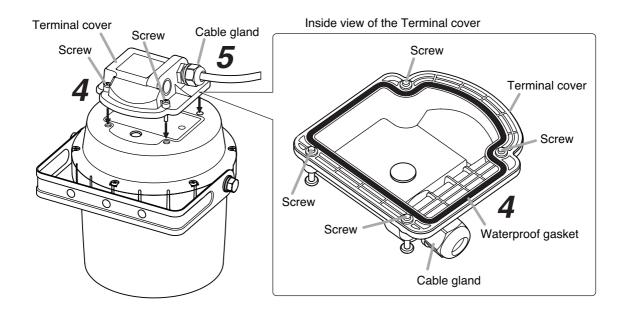
Step 5. Securely tighten the cable gland.
