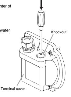
Step 2. Mount the cable gland to be added.
