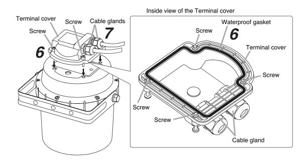
Step 7. Securely tighten the cable glands.
