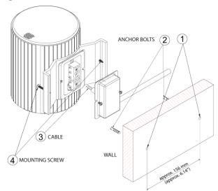
**Step 1.** Drill two holes in the wall or in the ceiling fitting with the anchor bolts supplied with the speaker.
